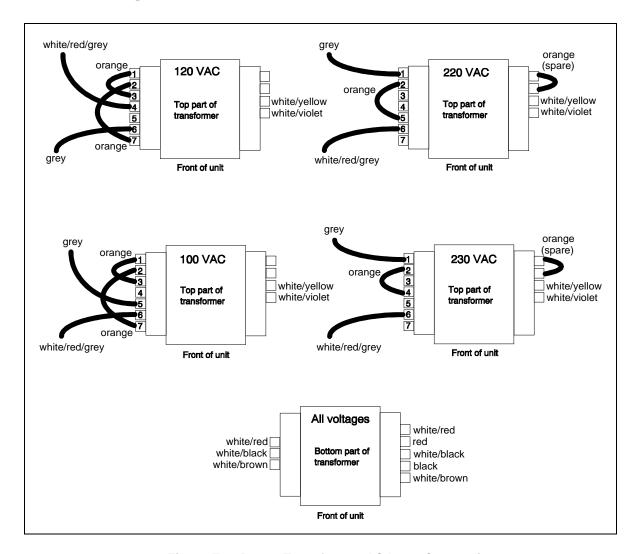
Figure E-1, Power Transformer AC Input Connections
